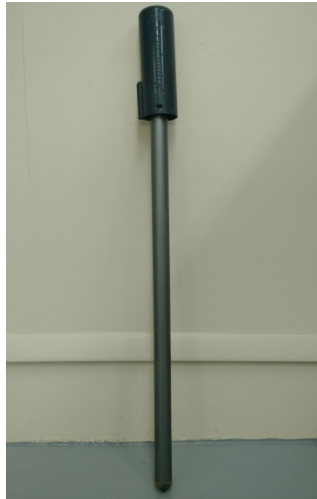
Figure 2. AquaCheck capacitance probe used for monitoring volumetric water content at each of the trial locations.
