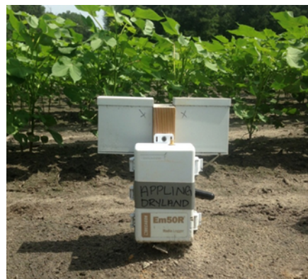
Figure 1. Decagon EM-50-R data logger and the tipping bucket rain gauges.
